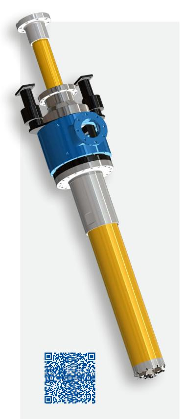
Depending on the intended purpose of the borehole, for instance, to support a bored diaphragm wall, or a subterraneous curtain wall, a cased drilling system is necessary to realise such a borehole. The system listed here features an external and an internal drill string, respectively, each driven independently by rotary head units that can also be moved in relation to one another.
