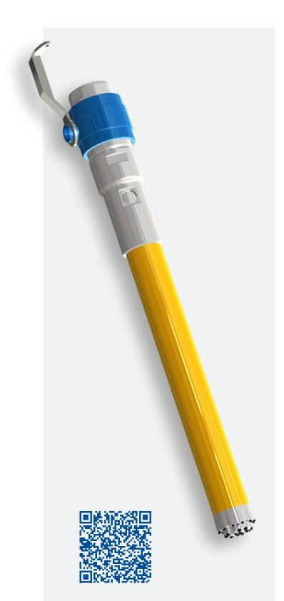
A method of drilling through the overburden with the aid of an outer casing to support the borehole wall is the so-called duplex drilling process. The system depicted here is drilled simultaneously with outer casings and inner rods and driven by a hydraulic drifter. The drill string thus experiences both rotation and percussion.
