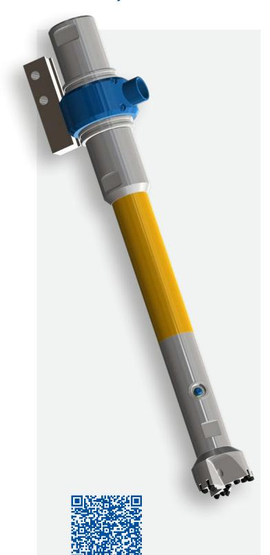
This drilling system is an erosion based system that creates in situ engineered geometries, such as columns, of mixed soil-cement in the subsoil. The aim is to improve the ground conditions by i. e. consolidation, vertical shoring or slicing the soil structure by means of a high velocity jet of grout at pressures of 100 bar (1450 psi) to 600 bar (8700 psi). The drill tools have been specifically designed to withstand these high pressures.
