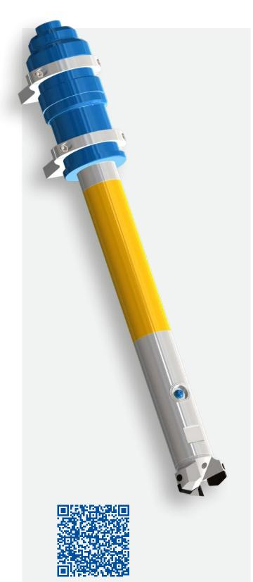
This drilling system is an erosion based system that creates in situ engineered geometries, such as columns, of mixed soil-cement in the subsoil. The aim is to improve the ground conditions by i. e. consolidation, vertical shoring or slicing the soil structure by means of a high velocity jet of grout at pressures of 100 bar (1450 psi) to 600 bar (8700 psi). The drill tools have been specifically designed to withstand these high pressures.
